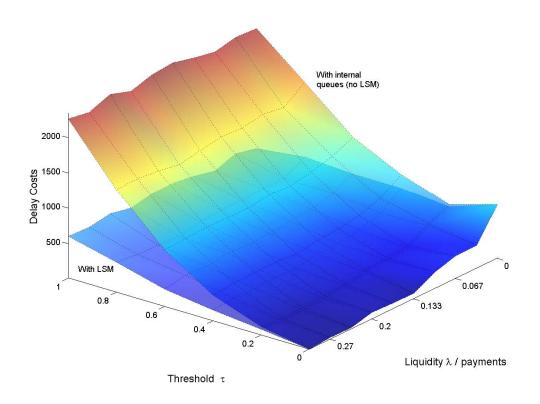
Figure 1: Delay costs for system with internal queues (top) and with LSM (bottom)
